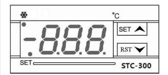
◆Relay and the compressor working state in the light
